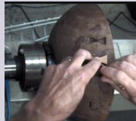
Inserting the bowtie & gluing it in. After it dries, he sands to close to the bowl's surface before returning the outside. The bow tie should not be visible from the inside because it needs strength of the bottom of the recess to achieve its purpose: holding the crack together.
