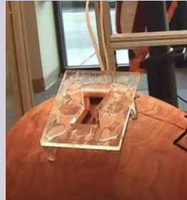
Here he is cutting the recess on a bowl. He hot glues the template to the bowl & cuts with the router. He used a chisle to make the corners sharp –straight in and levering out the corner.
