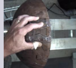
Gordon illustrated on a bowl –a recess for the butterfly & holding the template in place with hot glue
