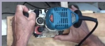
Cut insert with the router following the template by touch
