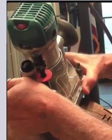
Here he is cutting the recess on a bowl. He hot glues the template to the bowl & cuts with the router. He used a chisle to make the corners sharp –straight in and levering out the corner.
