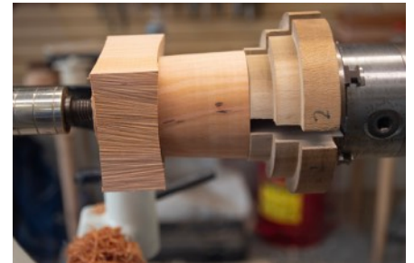
Shrink box mounted on special wooden chuck.
